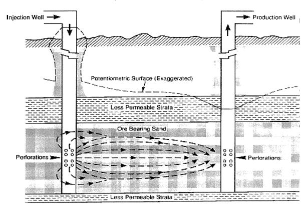
Figure 3. In situ leach mining process
